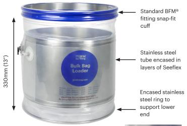
Pneumatic air inlet fitting connects to an air-line to inflate outer layer of Seeflex.
